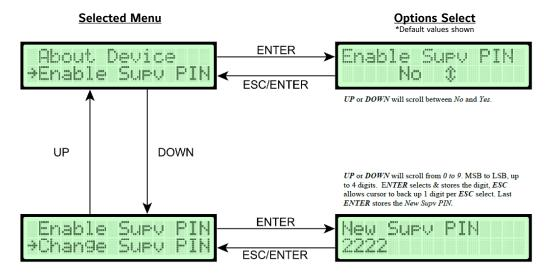
Note: The Supervisor Menu can be only accessed with a PIN, when enabled.
