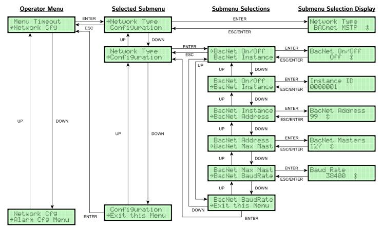
Firmware Note: Only ONE Network output configuration can be active at a time.
