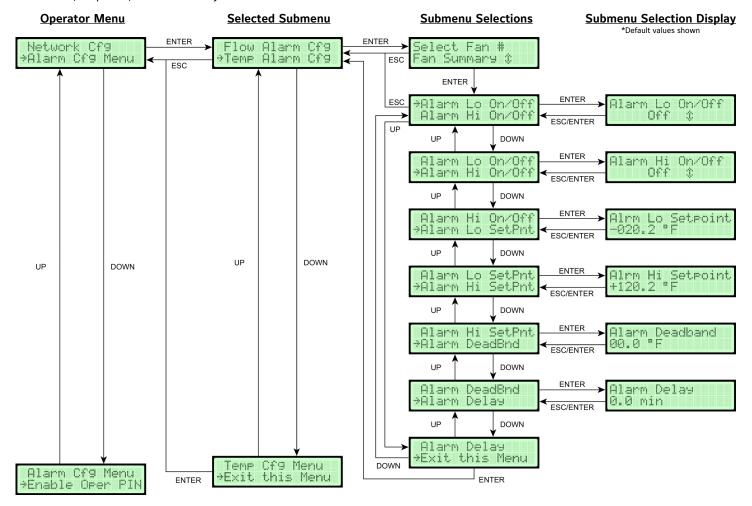
1. In the Operator Menu, press UP or DOWN to scroll to the RS-485 Interface Temperature Alarm Configuration submenu.
