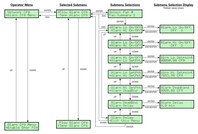
In the Operator Menu, press UP or DOWN to scroll to the RS-485 interface Flow Alarm Configuration submenu.
