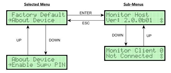
Use UP and DOWN to scroll through the possible connected devices on the monitor network to view the firmware version of each if they are connected.
