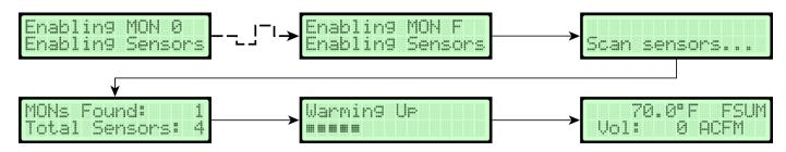
4. The TDFi-FA system will automatically reset all sensors and devices, then restart and warm-up. Then returns to the Normal Operational Mode.
