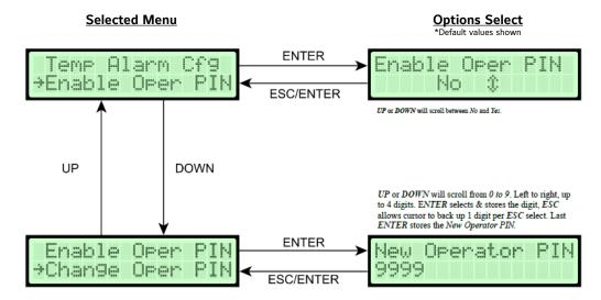
Note: The Operator Menu can be only accessed with a PIN, when enabled.
