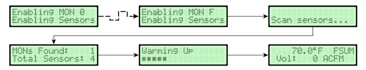
4. The TDFi-FA system will automatically reset all settings to default, all sensors, and devices, then restart and warm-up. Then returns to the Normal Operational Mode. All settings will be returned to a default state from the factory.
