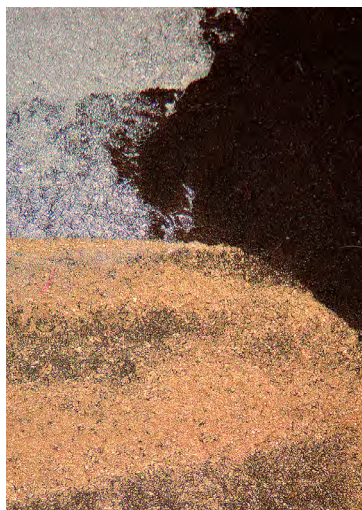
Fig. 91. Photomicrograph showing the metallic appearance and iridescent shimmer of lustrous pigments made by coating mica platelets with metal oxides or dyes. Field of view is approximately 7 x 12mm.
