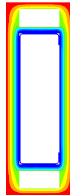
Figure 30 Temperature distribution of each column at 60 minutes under OZone fire_ Warehouse area _50%.
