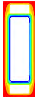
Figure 29 Temperature distribution of column at 60 minutes under OZone fire_Entire floor_100%.
