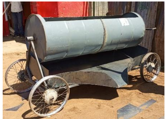
Figure 7a (above) and 7b (below): Two views of 2-barrel RoCC kilns in Kenya 2022
