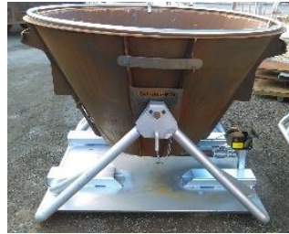
11.a) Wilson Biochar https://wilsonbiochar.com/ Ring of Fire ( far left) and 11.b) Terra Preta Developments https://www.terrapretadevelopments.com.au Kon-Tiki-Tas (near left). Both are Flame Cap (Cavity) kilns with open tops.
