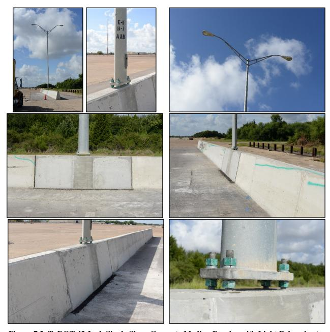
Figure 7.2. TxDOT 42-Inch Single Slope Concrete Median Barrier with Light Pole prior to Testing.
