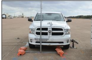
Figure 8.9. Skid-Mounted Single Perforated Steel Tube Temporary Sign Support System/Test Vehicle Geometrics for Test No. 468469-7-2.
