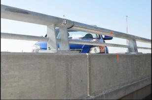
Figure 2.4. TxDOT C402 Bridge Rail/Test Vehicle Geometrics for Test No. 469468-1-1.
