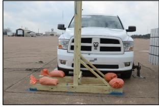
Figure 10.3. Skid-Mounted Dual Wood Post Temporary Sign Support System/Test Vehicle Geometrics for Test No. 469468-9-1.
