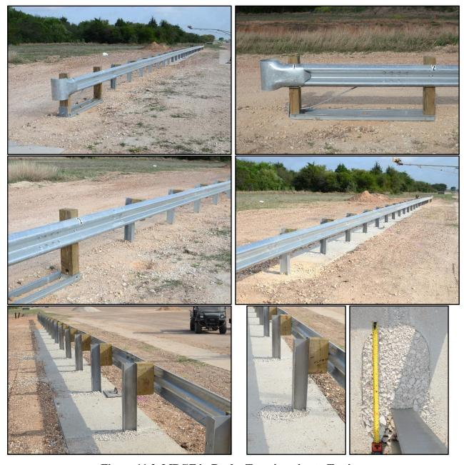
Figure 11.2. MBGF in Rocky Terrain prior to Testing.
