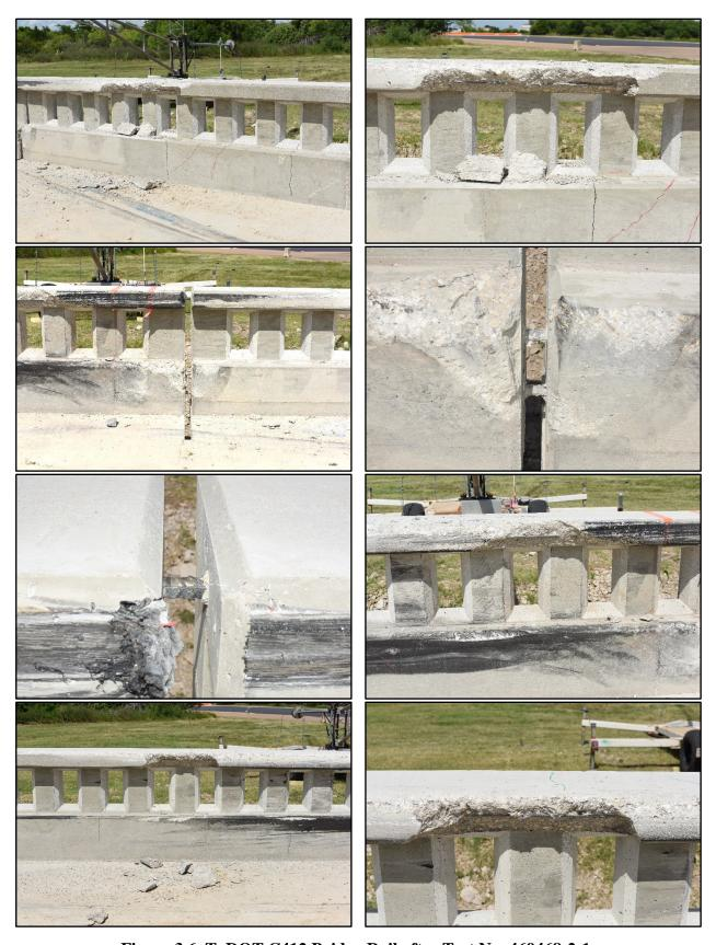
Figure 3.6. TxDOT C412 Bridge Rail after Test No. 469468-2-1.
