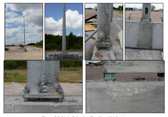
Figure 7.7. Light Pole after Test No. 469468-6-1.
