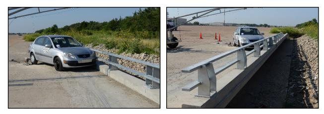
Figure 5.4. TxDOT T1W Bridge Rail/Test Vehicle Geometrics for Test No. 469468-4-1.
