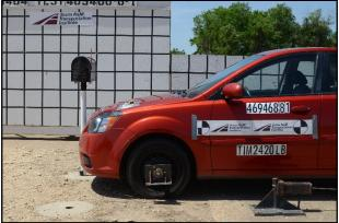
Figure 9.4. Single Mailbox with Recycled Rubber Support Post in Type 4 Foundation/Test Vehicle Geometrics for Test No. 468469-8-1.
