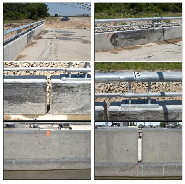
Figure 2.6. TxDOT C402 Bridge Rail after Test No. 469468-1-1.
