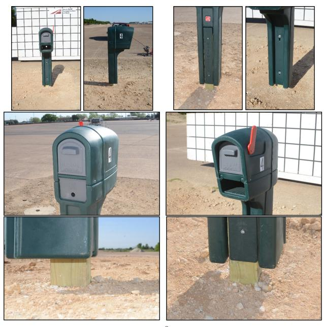
Figure 9.27. Single Molded Plastic Mailmaster® Mailbox with Wood Support Post in Type 5 Foundation prior to Testing.
