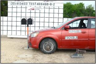
Figure 9.12. Double Mailbox with Thin-Wall Galvanized Support Post in Type 4 Foundation/Test Vehicle Geometrics for Test No. 468469-8-2.
