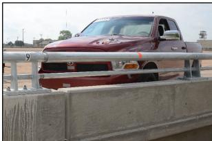
Figure 2.10. TxDOT C402 Bridge Rail/Test Vehicle Geometrics for Test No. 469468-1-2.
