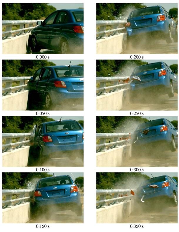
Figure A.2. Sequential Photographs for Test No. 469468-1-1 (Rear View).
