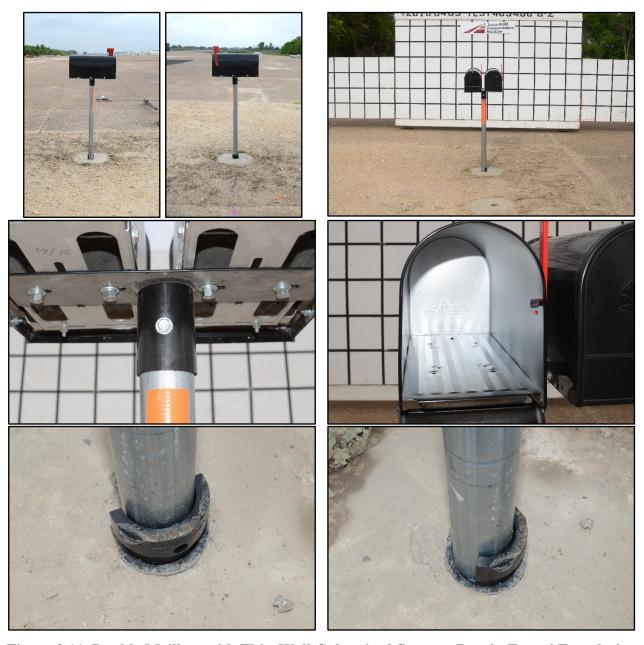
Figure 9.11. Double Mailbox with Thin-Wall Galvanized Support Post in Type 4 Foundation prior to Testing.
