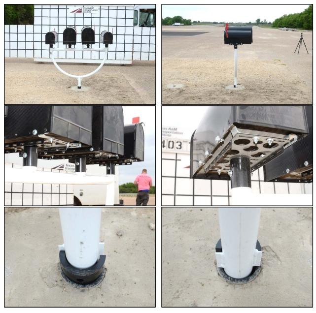
Figure 9.19. Multiple Mailboxes with Multi-Mount Support in Type 4 Foundation prior to Testing.
