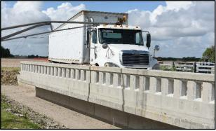
Figure 3.3. TxDOT C412 Bridge Rail/Test Vehicle Geometrics for Test No. 469468-2-1.
