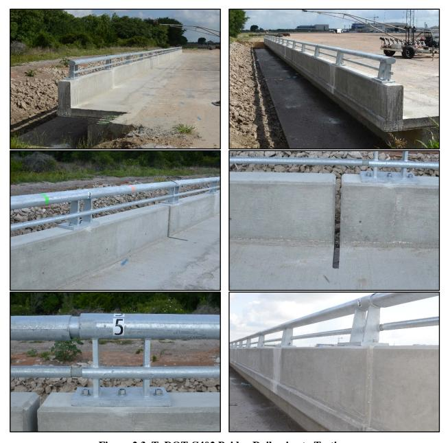
Figure 2.3. TxDOT C402 Bridge Rail prior to Testing.
