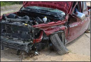
Figure 2.13. Test Vehicle after Test No. 469468-1-2.
