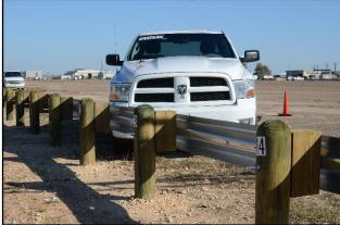
Figure 6.4. Round Wood Post W-Beam Guardrail/Test Vehicle Geometrics for Test No. 469468-5-1.
