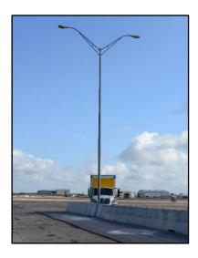
Figure 7.3. TxDOT 42-Inch Single Slope Concrete Median Barrier with Light Pole/Test Vehicle Geometrics for Test No. 469468-6-1.
