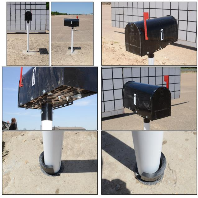
Figure 9.3. Single Mailbox with Recycled Rubber Support Post in Type 4 Foundation prior to Testing.
