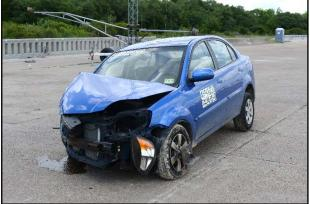
Figure 4.7. Test Vehicle after Test No. 469468-3-1.
