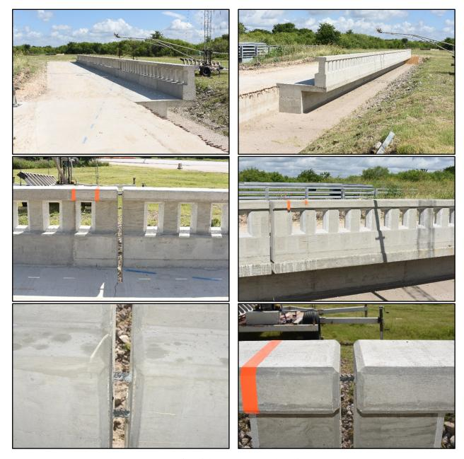
Figure 3.2. TxDOT C412 Bridge Rail prior to Testing.
