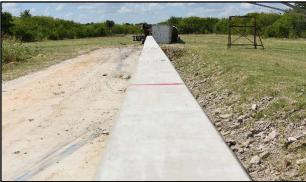
Figure 3.5. TxDOT C412 Bridge Rail/Test Vehicle after Test No. 469468-2-1.
