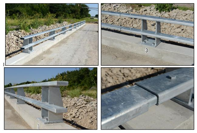
Figure 5.2. TxDOT T1W Bridge Rail prior to Testing.
