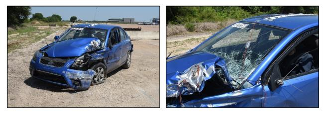
Figure 2.7. Test Vehicle after Test No. 469468-1-1.
