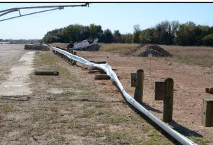
Figure 6.6. Round Wood Post W-Beam Guardrail/Test Vehicle after Test No. 469468-5-1.
