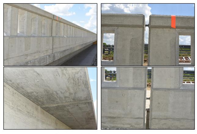
Figure 3.7. Field Side of TxDOT C412 Bridge Rail after Test No. 469468-2-1.
