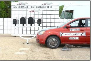
Figure 9.20. Multiple Mailboxes with Multi-Mount Support in Type 4 Foundation/Test Vehicle Geometrics for Test No. 468469-8-3.
