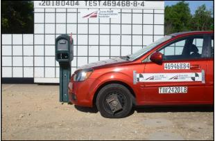
Figure 9.28. Single Molded Plastic Mailmaster® Mailbox with Wood Support Post in Type 5 Foundation/Test Vehicle Geometrics for Test No. 468469-8-4.
