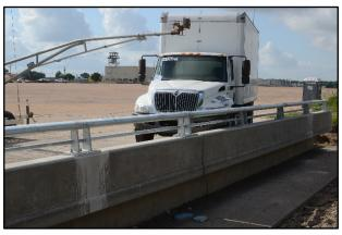
Figure 2.16. TxDOT C402 Bridge Rail/Test Vehicle Geometrics for Test No. 469468-1-3.
