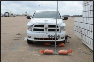
Figure 8.3. Skid-Mounted Single Perforated Steel Tube Temporary Sign Support System/Test Vehicle Geometrics for Test No. 468469-7-1.
