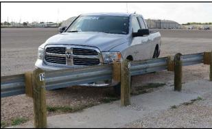
Figure 12.4. Round Post Guardrail/Test Vehicle Geometrics for Test No. 469468-12-1.
