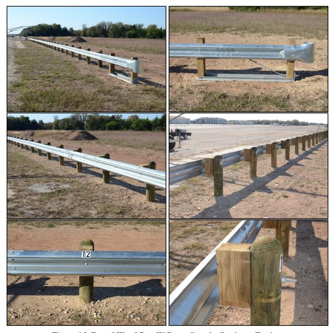
Figure 6.2. Round Wood Post W-Beam Guardrail prior to Testing.
