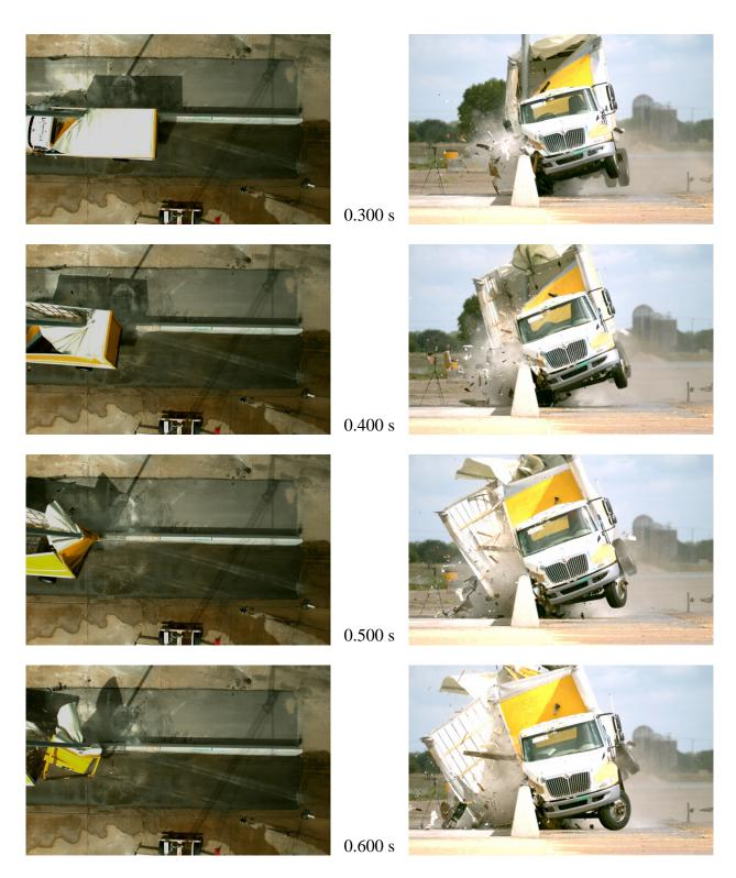
Figure F.1. Sequential Photographs for Test No. 469468-6-1 (Overhead and Gut Views) (Continued).
