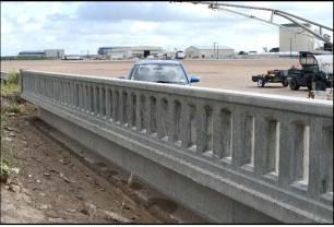
Figure 4.4. TxDOT C411 Bridge Rail/Test Vehicle Geometrics for Test No. 469468-3-1.
