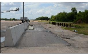
Figure 7.5. TxDOT 42-Inch Single Slope Concrete Median Barrier with Light Pole/Test Vehicle after Test No. 469468-6-1.
