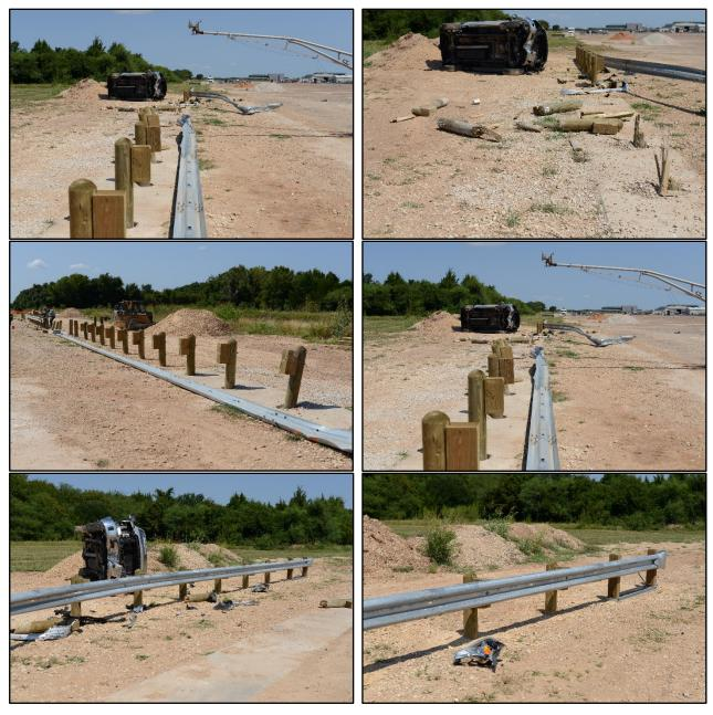
Figure 12.6. MBGF with Round Wood Posts in Rocky Terrain after Test No. 469468-12-1.
