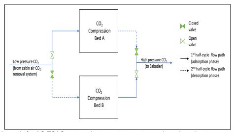
**Figure 1.** Schematic for AC-TSAC system that uses temperature swing adsorption to pressurize captured CO2 for processing.
