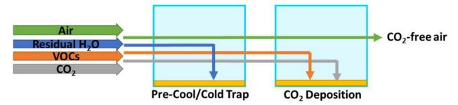
Figure 1. Basic Operation of the CDep system, cold surface represented by yellow block at base of box.
