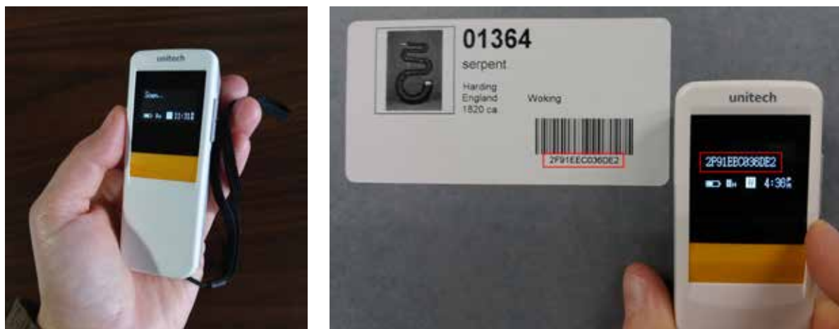
14. Pocket-sized barcode scanner MS926. The small OLED display on the scanner gives a quick reading of the last scanned barcode.
