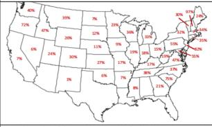
Figure 8: This map is based off of the event depicted in Figure 7, also from the High-Impact, Low-Frequency Event Risk to the North American Bulk Power System Report (June 2010). The map shows the "At-Risk EHV Transformer Capacity by State," with higher percentages indicating areas where power outage could last multiple years.
