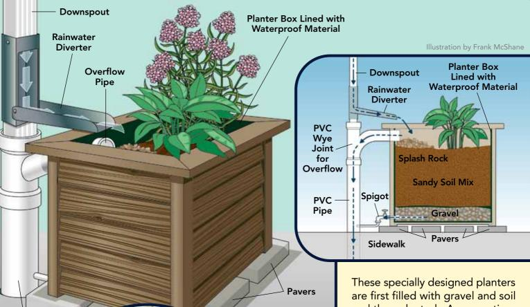
are first filled with gravel and soil and then planted. A connection to the roof downspout lets rain flow in and water the plants. There is another pipe that connects back to the existing downspout to drain excess water. These planters
