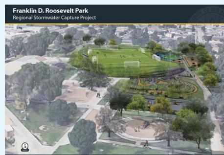
**The proposed Franklin D. Roosevelt Park Regional Stormwater Capture Project plans to divert dry- and wet-weather flows from the Glen Avenue Drainage System and to provide pretreatment of water for infiltration to the groundwater basin.**
