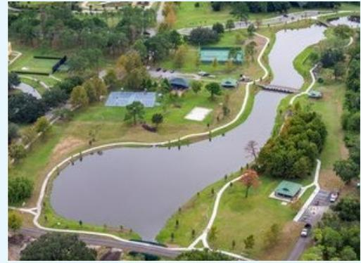
*Aerial view of the Lake Lawne Stormwater Reuse Facility, which uses captured stormwater to irrigate adjacent greenspaces.*
