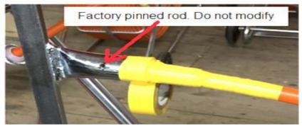
**Important to note:** The yellow tape is only in **place** during modification. Tape isn't required once the rod has been modified by the manufacturer.
